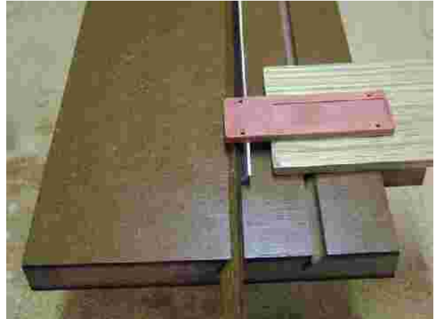
Shop made jig for sharpening planer blades using a diamond sharpener
